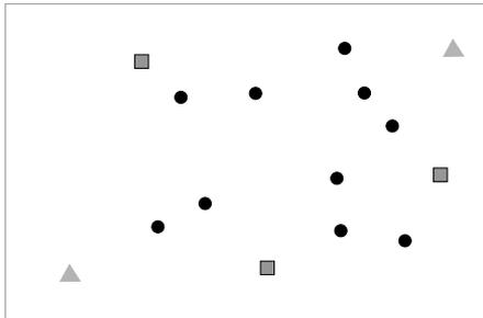
Again, if you were to perform this survey with a conventional total station, you would design a traverse plan which produced a strong looking network of closed-loop traverses through the points of the survey. *Fig. 4* shows one possible network design.
