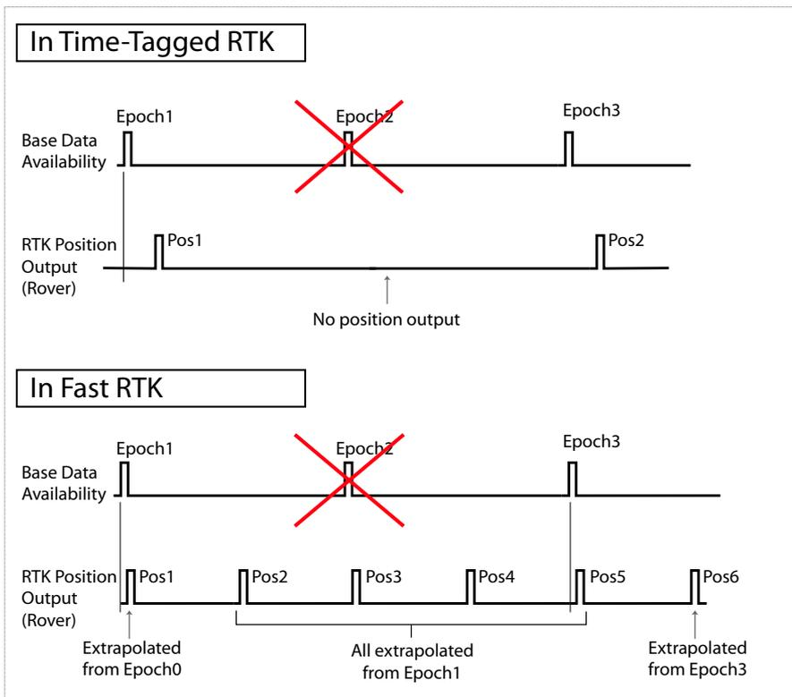
In the above Fast RTK mode example, the output rate has been set to twice the base data output rate.
