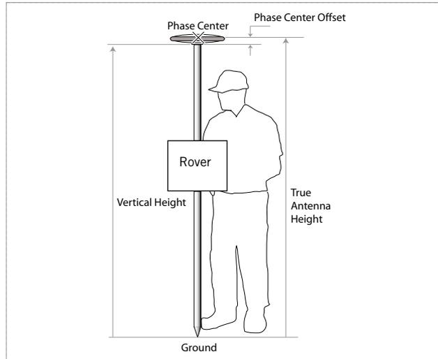
The real height of the antenna is therefore the sum of the vertical height and the phase center offset.
