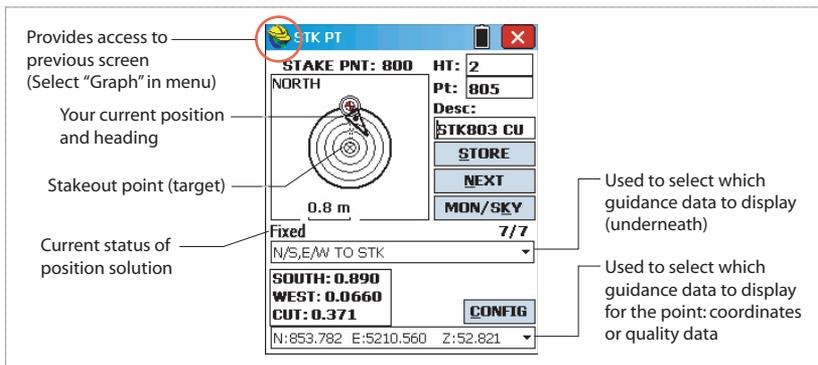
When the remaining distance is within the stakeout tolerance (this parameter can be changed in **Equip>Tolerances**), markers appear in the four corners of the target. You can now set a stake on this point.
