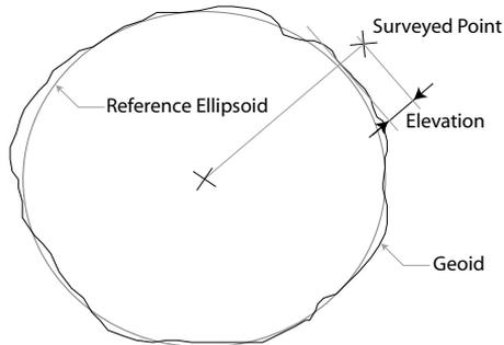
This surface is irregular depending on the density and distribution of materials on the surface of the Earth, which means the geoid may not exactly follow the natural features on the Earth's surface. (The geoid is a fictitious surface that can't be seen).
