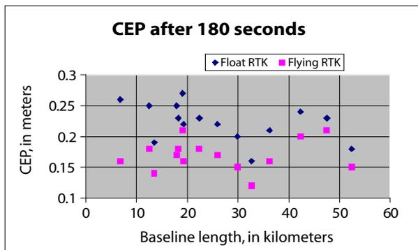
Again, L1 GPS-only data were used for evaluation. The plot shows that, even for long baselines, with only L1 GPS data, Flying RTK can deliver decimeter-level performance.
