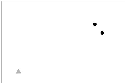
If you were to perform this survey with a conventional total station, you would probably plan on running a closed-loop traverse from the existing control point through the two new points (see *Fig. 2*). The same philosophy can be used for GNSS surveys. The figure below is your network design for this survey
