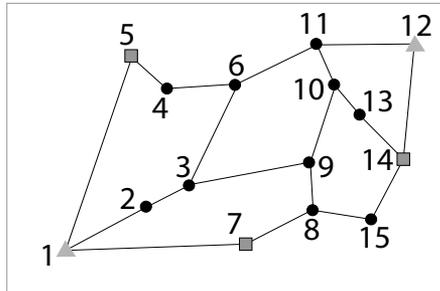
To execute this network design, you must perform a direct GNSS observation between all points directly linked. Each link can be viewed as a required vector. Counting the links in this network design, you will find that 19 vectors are required to execute this design.
