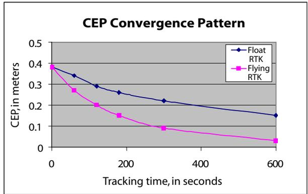
The CEP error (50% horizontal) is plotted vs. the time elapsed after BLADE was reset. The collected data include more than 150 reset operations for each of the different 22 baseline lengths used, which ranged from several meters up to ten kilometers.
