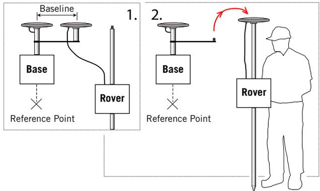
The Initializer Bar method can be used more especially when the survey takes place in the vicinity of the base (short baseline). It makes use of an initializer bar, also called
