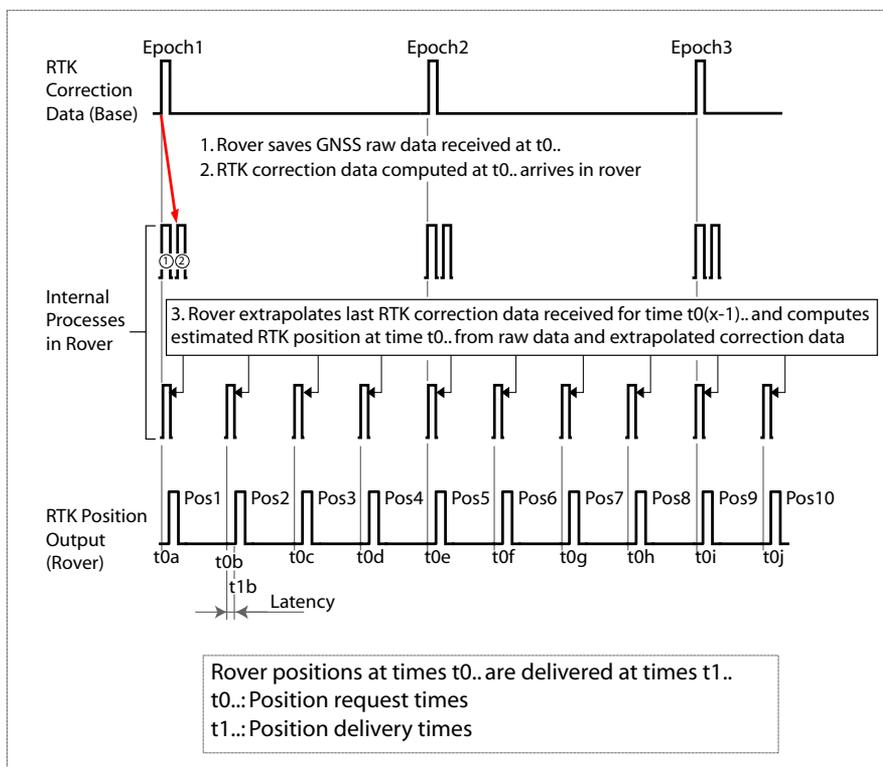
The time when position is requested is  $t_0$  and the time when the rover starts providing the position for time  $t_0$  is  $t_1$ . Times  $t_0a$ ,  $t_0e$  and  $t_0j$  in the base and the rover are synchronous because they originate from the same clock which is the GNSS time.
