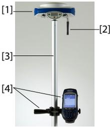
Mount the different items as shown on the picture, including the ProMark 500 [1], the radio antenna [2], the range pole [3] and the field terminal with its mounting bracket [4].
