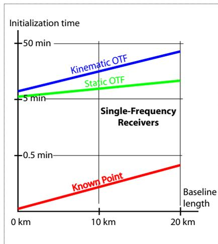
For single-frequency receivers using the initializer bar (baseline length: 20 cm), the TTFF is less than 60 seconds when one or more SBAS satellites are in view and their collection data are available.
