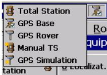
During a FAST Survey session, you can quickly change the receiver you are communicating with (provided the receiver you want to communicate with is within Bluetooth range).
