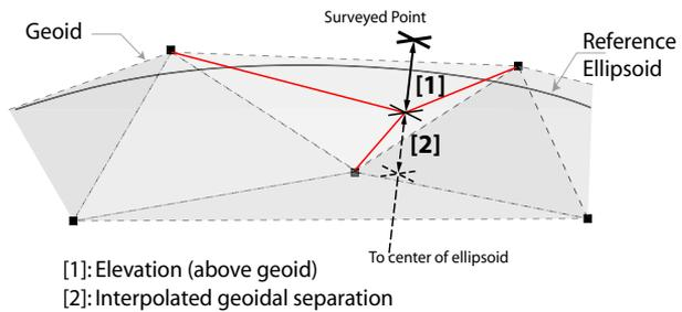
From this interpolation the system can derive elevation from ellipsoidal height using the following formula:
