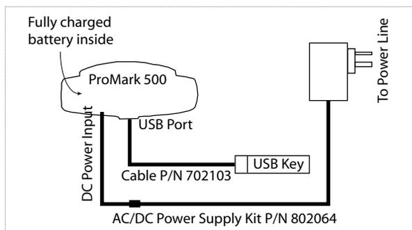
6. Connect the USB key now containing the upgrade files to the receiver's USB connector through cable P/N 702103 (provided).
