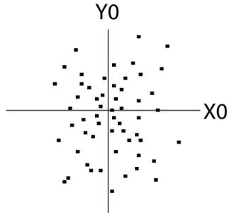
The origin of the (X0, Y0) axis system is the true position of the reference point. Each dot represents a position solution delivered by the GNSS System for this point.
