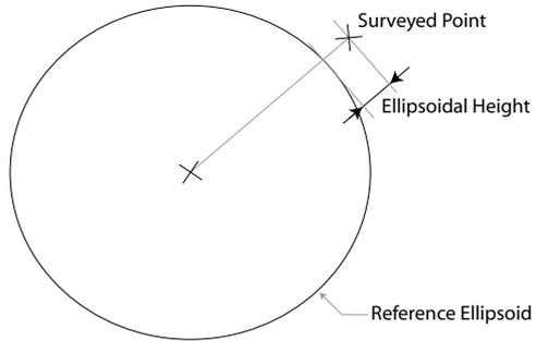
For a long time, surveyors have used the concept of “mean sea level” to measure the *elevations* of their points. The mean sea level was the common “zero” elevation. But this concept has shown some limitations.
