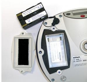
The battery used in the ProMark500 is a 7.4-V DC - 4400 mAh rechargeable battery. It is a standard model used in many camcorders.
