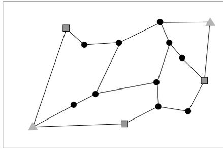
Although this network design was produced with conventional traversing in mind, this same design can also be used if performing the survey with GNSS equipment.
