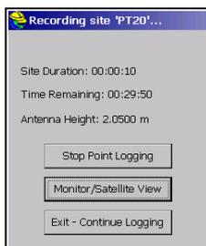
7. Tap on the **Monitor/Satellite View** button to make sure GNSS reception is good at the survey point (enough satellites are received, DOP values low). Ignore all RTK-related indicators.
