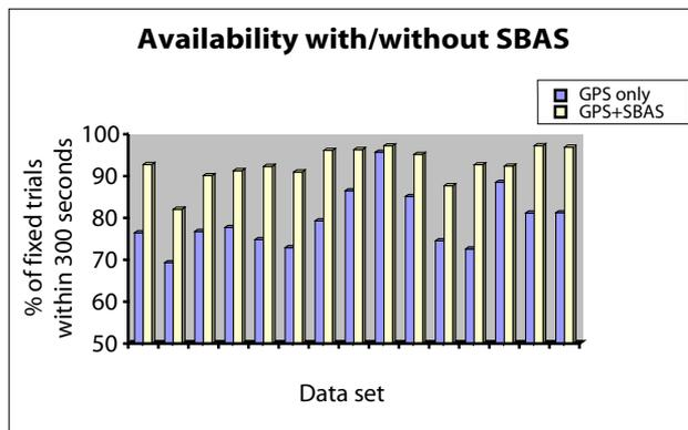
Using SBAS ranging in BLADE, the improvement is even more dramatic when processing baselines under medium/heavy shading. SBAS satellites noticeably improve geometry and result in dramatic improvement in performance over the GPS-only case. The first two data sets correspond to medium sky shading, while the third one corresponds to heavy shading where a GPS-only solution is typically useless.
