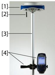
As a standard feature, the ProMark 500 incorporates a built-in GSM modem, which means you only have to connect the GSM antenna if you have paid for activation of the hardware. Mount the different items as shown on the picture, including the ProMark 500 [1], the GSM antenna [2], the range pole [3] and the field terminal with its mounting bracket [4].
